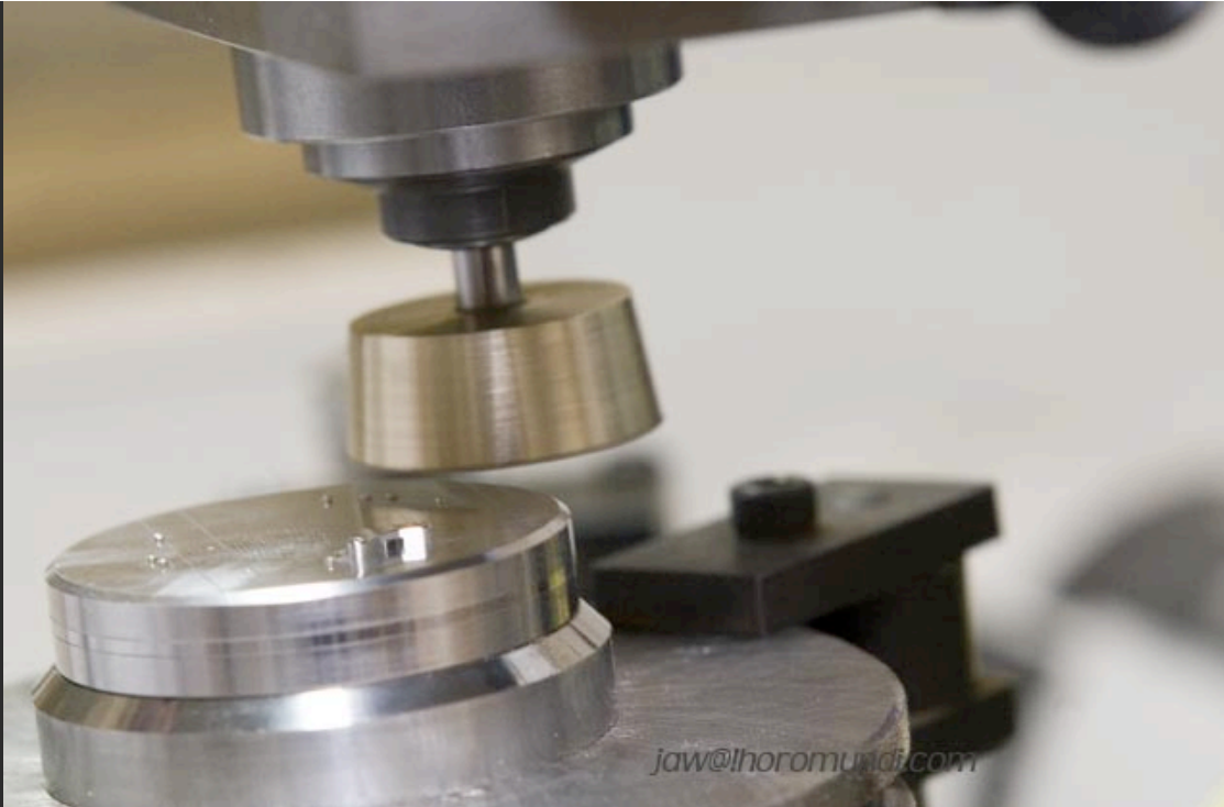
Hand operated automatic geneva stripping tool.
