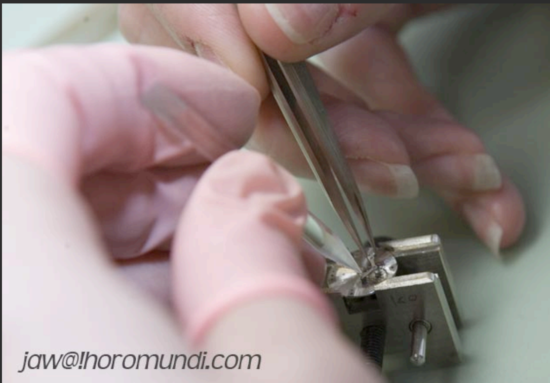
jaw@!horomundi.com The Central Tourbillon movement was the only automatic winding Central Tourbillon composed of 320 movement parts. It is also the only flying Central Tourbillon which has been COSC Chronometer certified, according to Omega.
