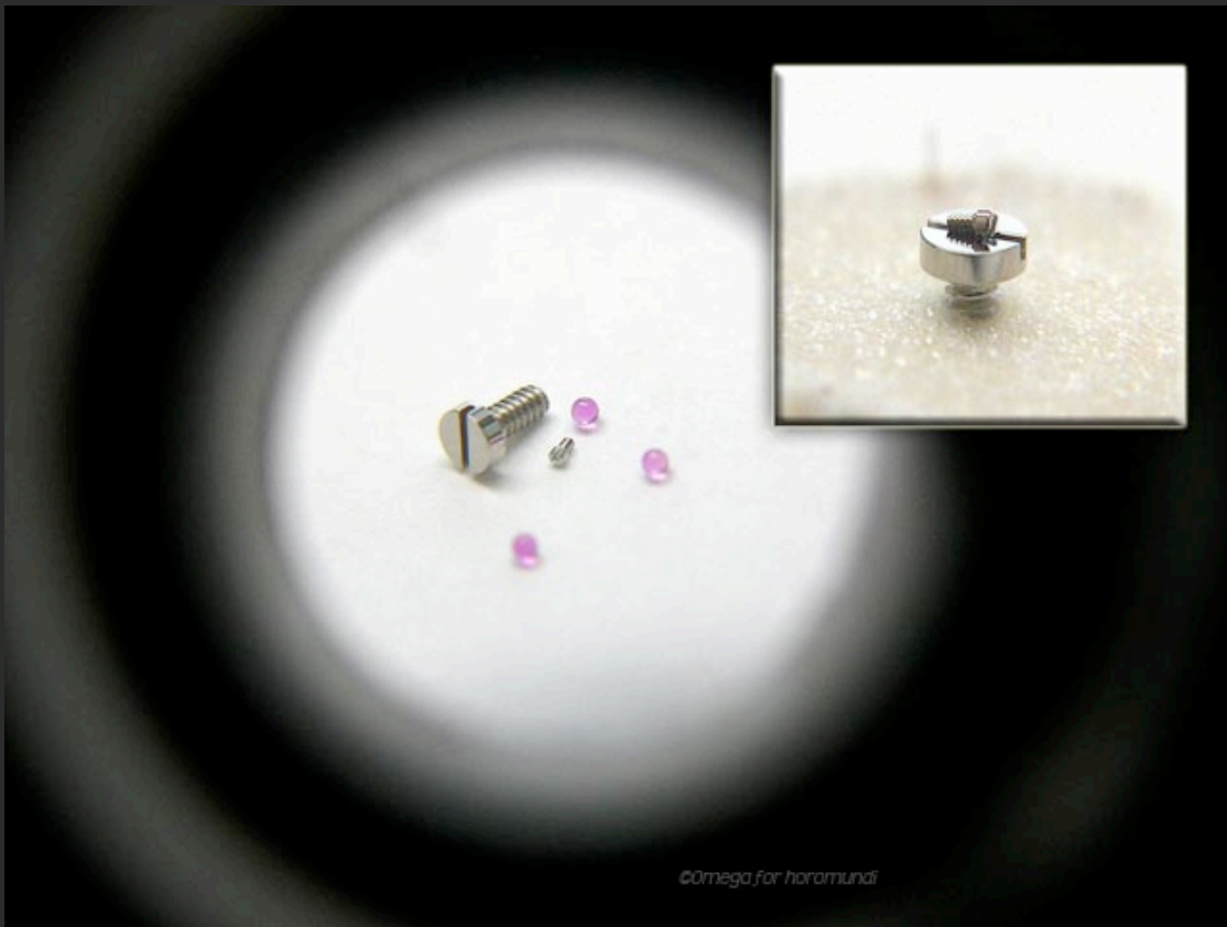
The relative sizes of a regular small screw and the minute stud screw.
