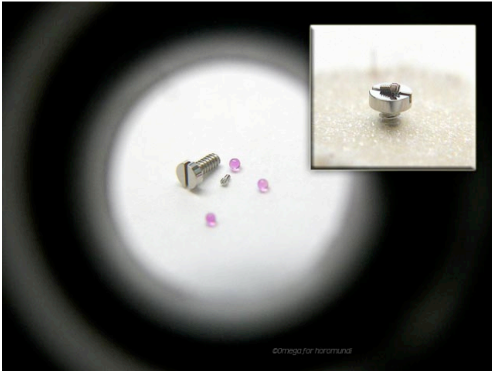
The relative sizes of a regular small screw and the minute stud screw.
